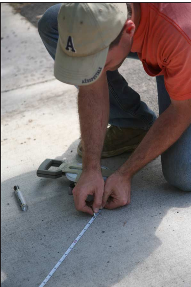
Curt takes a distance reading from the reference point out on the sidewalk. The readings are taken to an accuracy of one hundredth of an inch.
