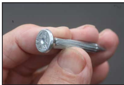
One of the concrete nails used to mark reference points in surveying.
