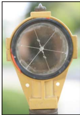
A close-up view head-on into the prism pole reveals the prism divided into six segments.
