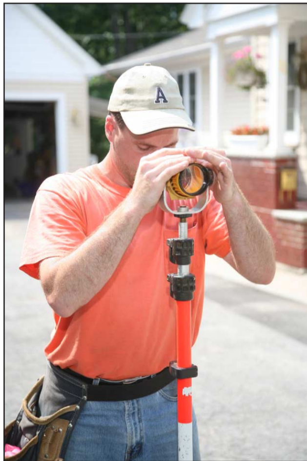
Curt is looking down to observe a bubble level, making sure that he is holding the prism pole exactly vertical while a reading is being made from the Total Station.
