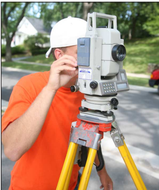
Rich operates the Total Station, which consists of a level, a theodolite (which gives angular measurements), and an EDM, which provides an electronic distance measurement.
