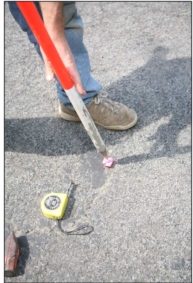
Curt places the Prism Pole into the indentation of the masonry nail.
